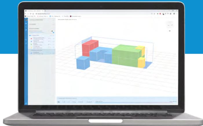
The 3D visualisation of the load and the ability to work with own load and vehicle dimensions allow for saving time required for the calculations. Sending a completed project to another person accelerates the loading process and minimises the risk that something will not fit in. If the entire space is not loaded, **Goodloading will suggest other spaces (trucks or containers) that will be suitable for the loads. Choosing a smaller vehicle usually generates lower costs.**
